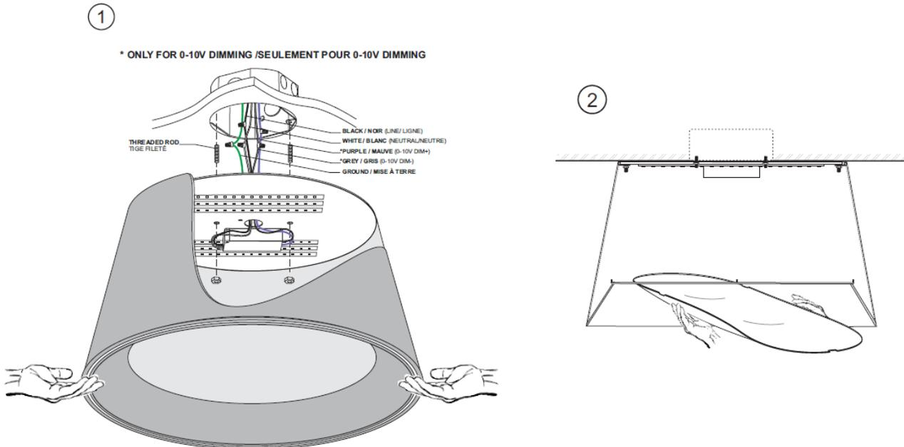
1. Make the electrical connections in the junction box. Secure the shade's mounting metal plate to the junction box with the 8-32 x 1" (2) threaded rods supplied with the luminaire.
