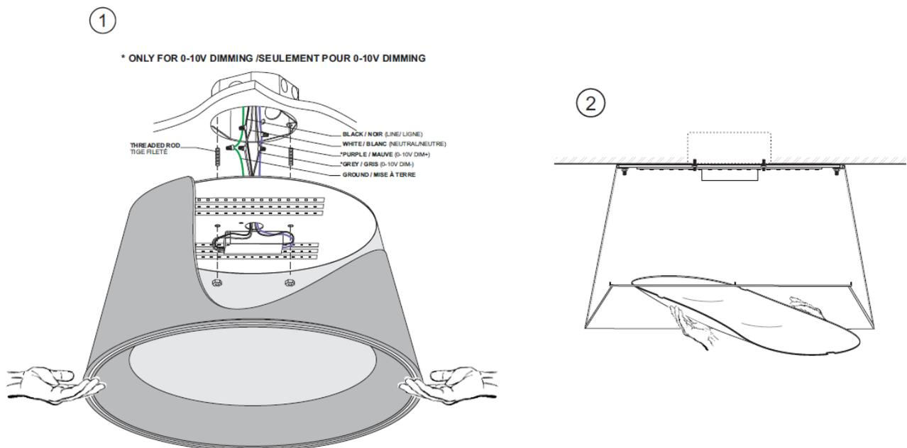
1. Make the electrical connections in the junction box. Secure the shade's mounting metal plate to the junction box with the 8-32 x 1" (2) threaded rods and nuts supplied with the luminaire. Secure the mounting plate to ceiling by using 4 screws (supplied by others). Make sure to have sufficient reinforcement for the anchoring screws.
