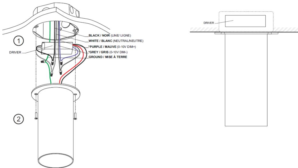
1. Connect the electrical wires in the deep junction box (supplied by others).
