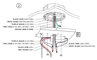
\*ONLY FOR 0-10V DIMMING / SEULEMENT POUR GRADATION 0-10V
