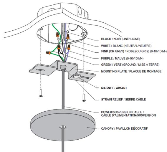
1. Connect the luminaire's electrical wires to the electrical J-box's wires. **\*\*\*For phase dimming, leave pink (or grey) and purple wires as is. Do not connect them together nor to any other wire.**
