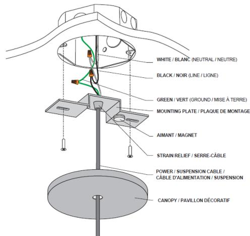
1. Connect the luminaire's electrical wires to the electrical J-box's wires.
